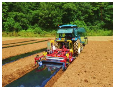
Figure 4. A Machine applying soil disinfection film in the field.
