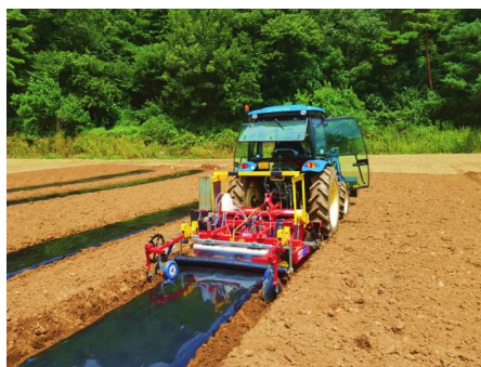
Figure 4. A Machine applying soil disinfection film in the field. https://www.researchgate.net/figure/Soil-disinfection-machine-used-in-this-study_fig1_349317572
