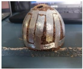
Figure 1. Side view of the coconut shells in the rain sensor
